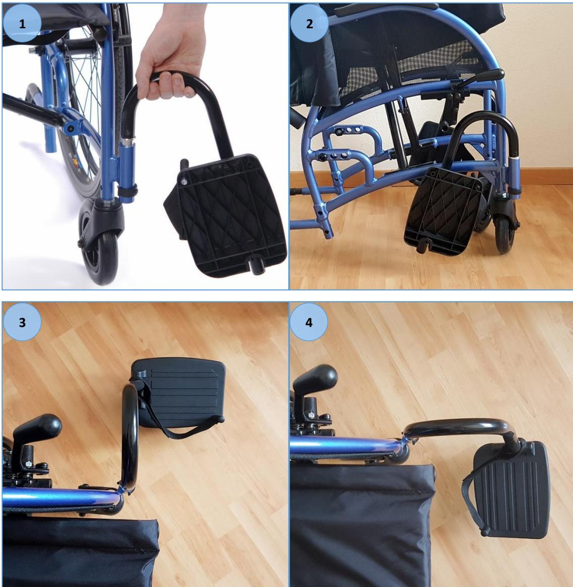
The lateral locked position is only intended for use when the user of the wheelchair is getting in and out of the chair. The chair should not be moved with the footrests locked in this position as the footrests may get caught on an obstacle or obstruction.
