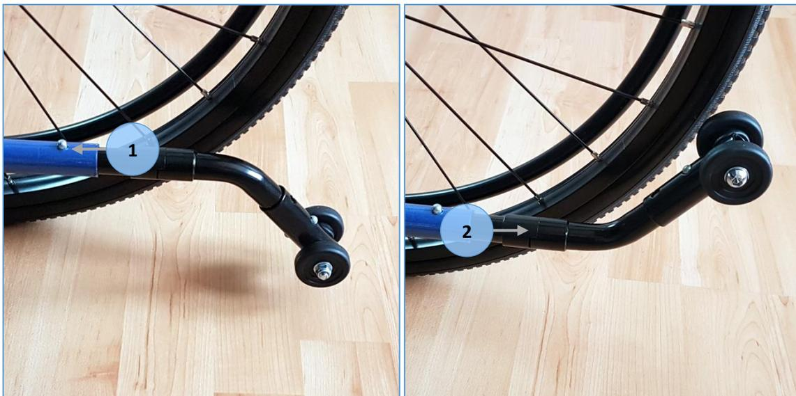
If the wheelchair is to go up or down a high step (e.g. a curb), the anti-tip wheels must be swiveled upwards to avoid them catching on the ground. Pull on them to unlock (2) and swivel up/down so it looks like picture 2 above.
