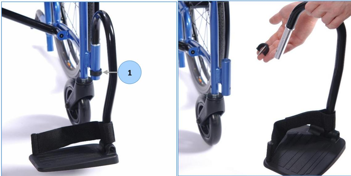
The footrests can be completely removed from the wheelchair by pulling the plastic clip with its retaining pin (1) horizontally out of the tube. The whole of the footrest can then be pulled up and out of the footrest mounting. When refitting the footrests ensure that the hole for the locking pin in the footrest is aligned with the hole in the frame.
