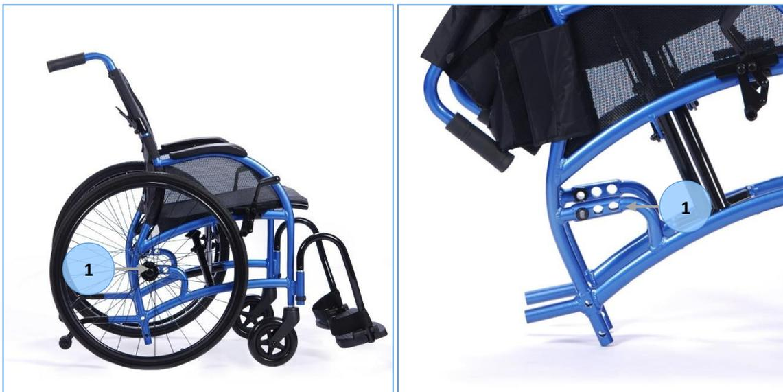
The further back the axle mounts are installed, the less likely the wheelchair is to tip over in use, i.e. in this configuration there is the least likelihood of the wheelchair tipping backwards. The further forward the axle mounts are installed, the lower the proportion of the total weight that is over the forward casters, making it easier to deliberately tip the wheelchair backwards (either by the user or the companion), which in turn makes the chair easier to maneuver.
