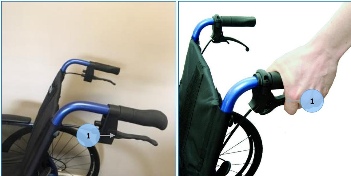
The attendant brakes can be locked in one of the following two ways (depending on the type of attendant brake installed on your wheelchair):
